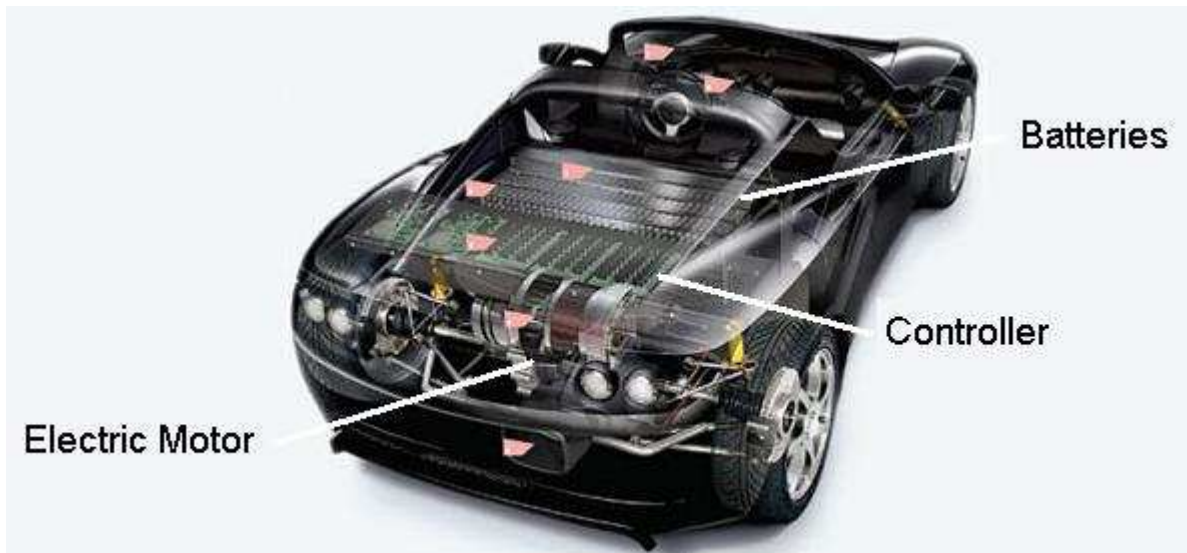
Figure 1: The Basic Components of an Electric Car
